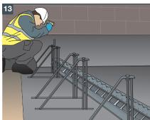
Pin ArmourFix jacks into place.
