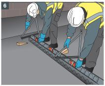
Fit ArmourFix jacks to the ShieldJoint with ShieldJoint jack fittings (these can be ordered separately).
