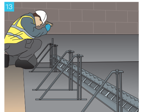
Pin ArmourFix jacks into place. Do not use pin and welding installation method as it may result in misalignment of the joint.
